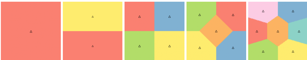
Figure 7: Plot of the Lloyd’s centroidal power diagrams for n = 1, 2, 4, 5, 7 cells from left to right. The sites coincide with the barycenters of the cells.
